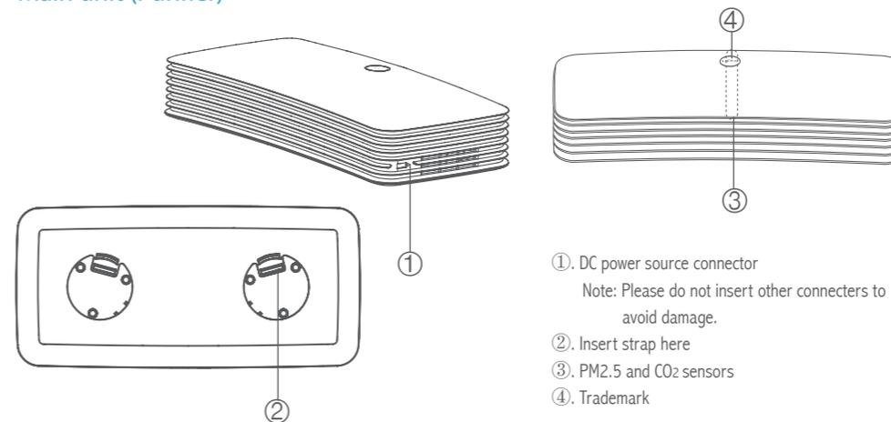
**NOTE:** Do not block the air inlet and outlet as the PM2.5 and CO<sub>2</sub> sensors are located in the center of the purifier.
